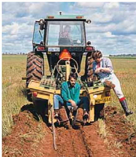
Photo 5.10. Planting saltbush seedlings with a commercial tree planter
